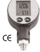
LEO 2 is a compact, micro-processor ( $\mu$ P) controlled, highly accurate and versatile pressure measuring instrument with digital indication. The piezoresistive pressure transducer as the heart of the instrument has gone through extensive pressure- and temperature tests. Its characteristics are
